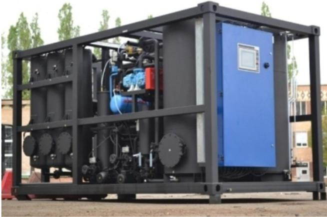
The purpose of transformer oil reclamation is extracting moisture, acids, mechanical dirt and undesirable components such as unsaturated hydrocarbons, asphalt-resinous substances, sulfur and nitrogen compounds. For the reclamation of waste oils used various technological operations, based on the physical, physico-chemical and chemical processes.
